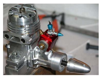
**SMALL DIESEL!** Wait, take a closer look. That's a 60 size glow engine with the small diesel almost swallowed up in the carburetor.
