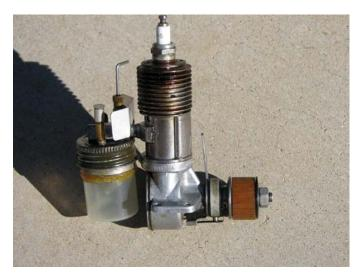
Here's that Brown junior exhaust deflector mentioned earlier. It doesn't restrict exhaust flow nor cause hot running as did those restrictive little clamp-on exhaust pipes. It's held on by the spraybar and has extended "legs" down around the intake tube to prevent rotation.
